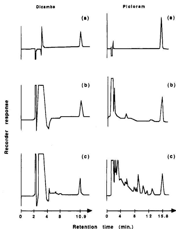
Figure 1. Examples of chromatographs for dicamba and picloram: (a) 500 ppb standards; (b) solutions that were passed through SPE cartridges; (c) solutions that were recovered from soil samples.
